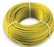
01840.Y Bus buglar alarm system cable, halogen-free 2x0,50 mm 2 , rated operating voltage to earth 400 V, suitable for I category cables, yellow - 100 m
