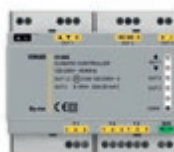
■ 01465 Climate control device for heating systems, 120-230 V~ 50/60 Hz, 3 inputs for PT100, PT1000 and NTC probes, 1 output for mixer valve, 1 output 0-10 V or (0)4-20 mA, 1 change-over relay output 8 A 230 V~
