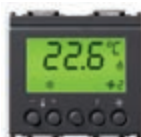
■ 16915 Thermostat for ambient temperature control of 2 independent zones (heating and air-conditioning), KNX standard, NO 4 A 24 V~ relay output + 1 temperature sensor input + 1 programmable input - 2 modules
