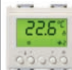
■ 16915.B Thermostat for ambient temperature control of 2 independent zones (heating and air-conditioning), KNX standard, NO 4 A 24 V~ relay output + 1 temperature sensor input + 1 programmable input - 2 modules
