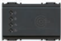
■ 16927 Transponder card reader for installation outside rooms, KNX standard, 2 NO 4 A 24 V~ relay outputs, 2 inputs, power supply 12-24 V~ 50/60 Hz and 12-24 Vdc (SELV) - 3 modules. Supplied without transponder card
