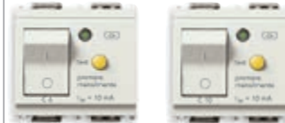
16511.06.B C 6, I_{\Delta n} 10 mA, breaking capacity 1500 A - 2 modules 16511.10.B C 10, I_{\Delta n} 10 mA, breaking capacity 3000 A - 2 modules
