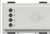
■ 16927.B Transponder card reader for installation outside rooms, KNX standard, 2 NO 4 A 24 V~ relay outputs, 2 inputs, power supply 12-24 V~ 50/60 Hz and 12-24 Vdc (SELV) - 3 modules. Supplied without transponder card
