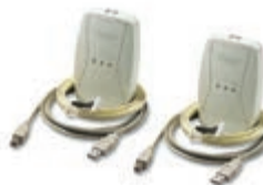
■ 01993 Hardware interface for programming By-me serial devices and Well-contact Plus touch screens and for configuring By-me systems
