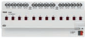
■ 01521 Actuator with 12 10 A 250 V~ 50/60 Hz relay outputs for fluorescent lamps, KNX standard
