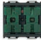
16966 2 rocker push buttons + 8 A 120-230 V~ change-over relay output actuator - 2 modules
