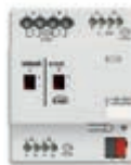
■ 01528 Dimmer, 2 inputs for 01530, 2 NO 16 A 250 V~ relay outputs, 2 1-10 V outputs, KNX standard
