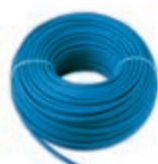
01840.B Cable for sound system, halogen-free 2x0,50 mm 2 , rated operating voltage to earth 400 V, suitable for I category cables, blue - 100 m
