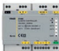
01465 Climate control device for heating systems, power supply 120-230 V~ 50/60 Hz, 3 inputs for PT100, PT1000 and NTC probes, 1 mixer valve control output, 1 0-10 V or (0) 4-20 mA output, 1 16 A 230 V~ change-over relay output
