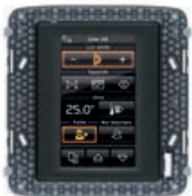
Δ 20848.1 Color touch screen, 4,3", for the control, 1 temperature sensor input, with built-in mounting frame for installation in 8-module mounting box. Depth: 39,9 mm
