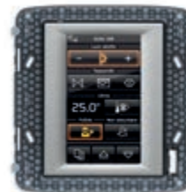
Δ 20848.1.N Color touch screen, 4,3", for the control, 1 temperature sensor input, with built-in mounting frame for installation in 8-module mounting box. Depth: 39,9 mm
