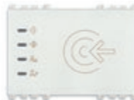
■ 19457.B Transponder card reader for installation outside rooms, KNX standard, 2 NO 4 A 24 V~ relay outputs, 2 inputs, power supply 12-24 V~ 50/60 Hz and 12-24 Vdc (SELV) - 3 modules. Supplied without transponder card
