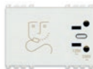
19290.B 230 V~ 50/60 Hz, with 20 VA isolating transformer, 230 V~ and 120 V~ outputs - 3 modules
