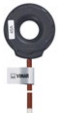
▲01458 Toroidal current sensor for load control and power measurement, hole diameter 19 mm, cable length 40 cm
